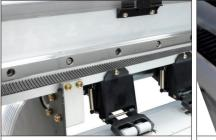
**Guide Rails**High-quality guide rails ensure stable printhead movement, high precision, low noise, and long lifespan.
