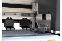
**Anti-collision sensor** When the cart touches a foreign object, the switchs will be on, and machine stops printing.
